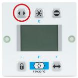
Pressing The Hold Open Button Twice Puts The Door To Manual Operation
