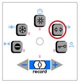
Press Once = Hold Open Press Twice (Flashing)= Manual Mode
